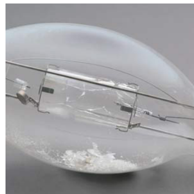
Ruptured arc tube contained within the intact outer jacket of a Venture MP lamp
